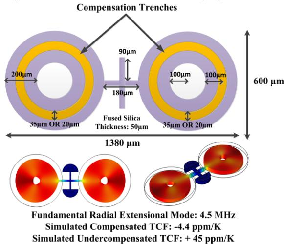
Figure 1: Sketch and simulated mode shapes for a fundamental radial extensional mode of the 50  $\mu\text{m}$  thick dogbone resonator. The nickel trench depth was chosen to be 30  $\mu\text{m}$ , with two chosen trench widths of 35  $\mu\text{m}$  and 20  $\mu\text{m}$ . The simulations assume a nickel TCE of -600 ppm/K.
