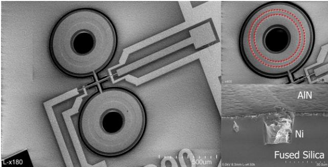
Figure 4: (Left) A SEM image of a fabricated temperature compensated dogbone resonator. (Top right) A zoomed SEM image of a dogbone ring with nickel compensation trench outlined in the center of the ring. (Bottom right) A cross-section SEM image of a nickel-refilled trench with a measured depth of 20  $\mu\text{m}$ .
