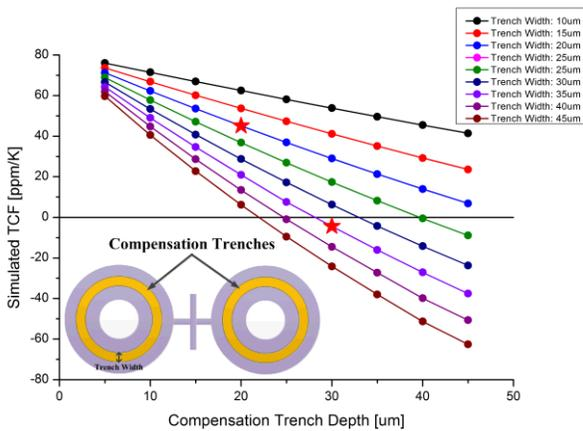
Figure 2: Simulated TCF results for dogbone resonators with varied compensation trench sizes. Starred data points are the selected trench depth/width combinations for the fabricated resonators. Nickel is assumed to have a TCE of -600 ppm/K.
