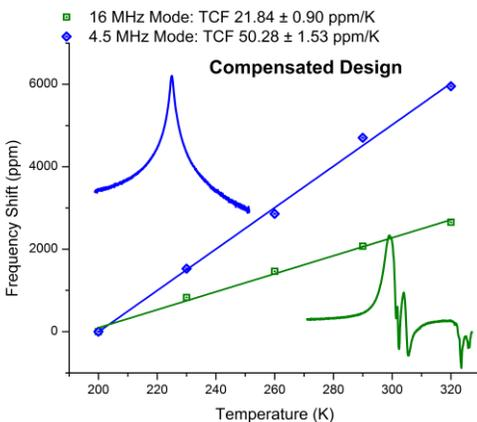
Figure 7: Measured TCF data comparing a compensated fundamental radial extensional mode with a higher frequency mode. A 28.5 ppm/K difference in TCF is seen between the two modes. Insets show the measured S-parameter response for each mode.
