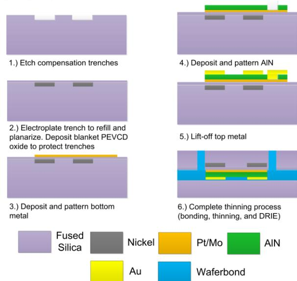
Figure 3: Fabrication flow for compensated fused silica resonators.
