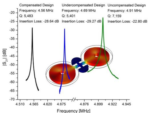
Figure 5:  $S$ -parameter response and measured parameters for a compensated, undercompensated, and uncompensated dogbone in the fundamental radial extensional mode. Background image shows the simulated mode shape.
